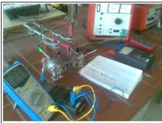
Figure.1 : Schematic symmetrical electrochemical cell made of Teflon , for voltammetric measurements
