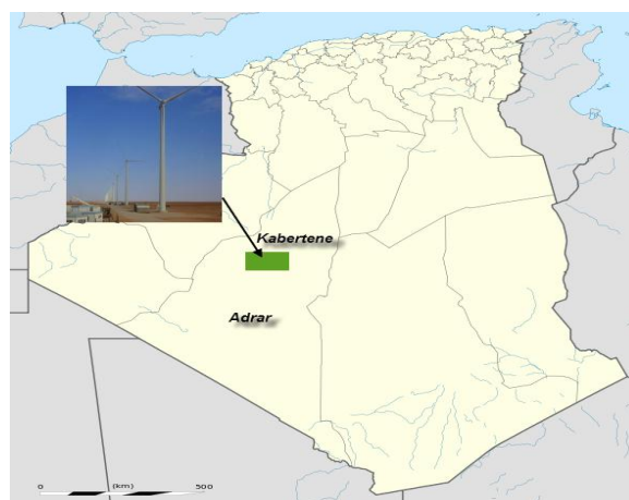
Fig.1. The new power generation central, first of its kind at national level, has a capacity of 10 megawatts, is located on a surface of 30 hectares in the zone of Kabertene, 72km north of the Willaya of Adrar. It is constituted by 12 wind turbines with an output of 0.85MW each.
